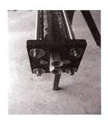
Insert the end plug assembly into the vessel end. Push the tie rods through the bearing plate and place a 316 stainless washer on each tie rod end.
