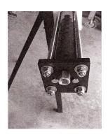
Screw 316 stainless lock nuts onto each tie rod. This is easily done by holding the lock nut with a wrench and turning the slotted tie rod with a flat head screwdriver. Do not over-tighten. Bring the lock nut just into contact with the washer. Repeat on other vessel end.
