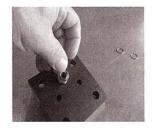
Place a spiral ring over the nose of the hex port, and, using a small flat head screwdriver, walk the ring into the grove on the hex port.
