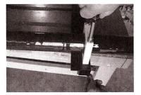
Place top half of mounting block on the vessel and mount to your frame.
